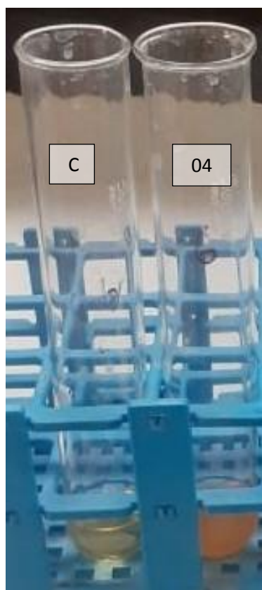
Figure 2. Analysis of Vanillin formed from FA biotransformation using TBA method. Note: C= control (bioconversion media without isolate 04); 04 = bioconversion media with isolate 04.
