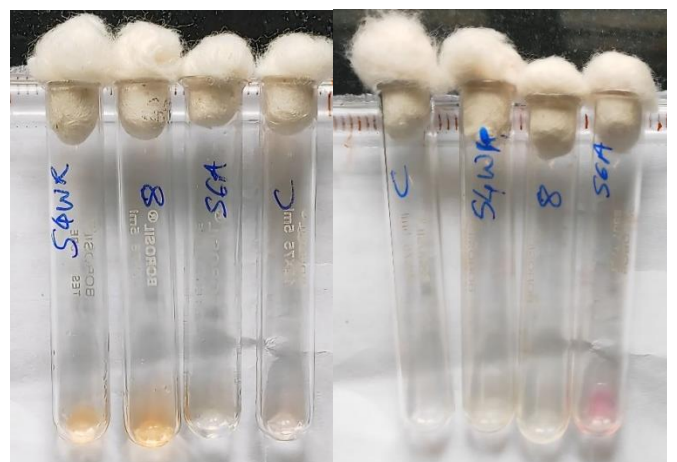
Figure 2. Hexane extracts of Isolate No. 8, and S4WR positive for phytosterol group (Left) and hexane extract of S6A positive for emodins (Right).
