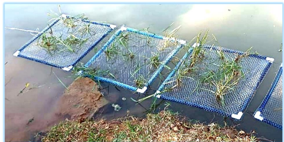
Figure 6. In-situ application of Vetiver grass and Bermuda grass using a floating treatment wetland in contaminated water for 30 days.
