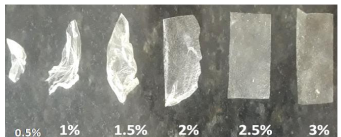
Figure 5. Bioplastic preparation from cellulose biomass in combination with 0.5%, 1%, 1.5%, 2%, 2.5%, and 3% of gelatin
